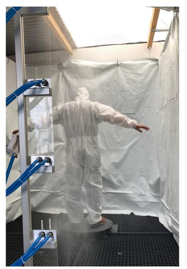
A chemical protective suit protects the person wearing it from chemicals in gaseous, liquid and / or solid state. They are classified into 6 types with different protection levels from gastight to restricted liquid-tight.
